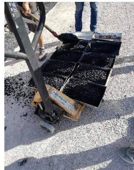
Fig.15. Collection of asphalt mixture for testing
