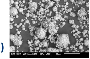
SEM morphology of antimicrobial additives: a) polylysine (PLY), b) polylysine immobilized on sodium montmorillonite (PLY/MM) and c) polylysine immobilized on aminedodecanoic acid intercalated on MMT (PLY/MM/ADA)
